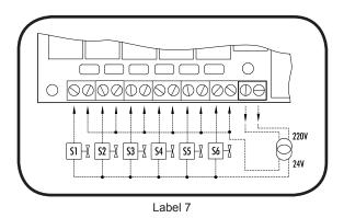
Also, pumps with different operating tension can be combined. Example: 5 pumps 220V  $\sim$  and 1 pump 24V  $\sim$ . (See Label 8)
